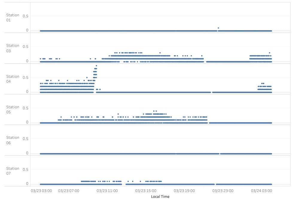
Preliminary Fixed Station Real-time Air Monitoring Readings PROJ-052216 | SPS Technologies Fire | Abington Township, PA 3/23/2025 4:02:45 AM to 3/24/2025 4:01:07 AM | **Analyte: LEL (%)**
