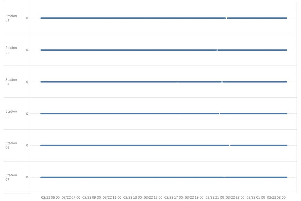
Preliminary Fixed Station Real-time Air Monitoring Readings PROJ-052216 | SPS Technologies Fire | Abington Township, PA 3/22/2025 4:03:32 AM to 3/23/2025 3:59:38 AM | **Analyte: HCN (ppm)**
