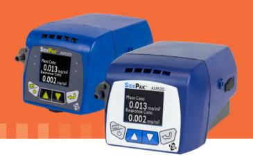
The SidePak™ AM520 and AM520i Personal Aerosol Monitors are small, portable, battery-operated, data-logging, light-scattering laser photometers that provide real-time aerosol mass concentration readings of dusts, fumes, mists, smoke and fog within a worker's breathing zone.
